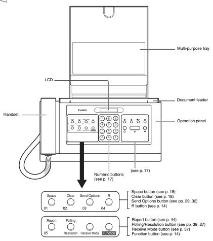
The buttons on the left of the operation panel have the following two functions:
